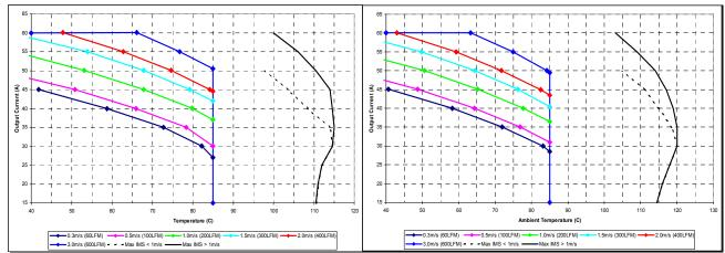
Maximum output current vs. ambient temperature at nominal input voltage for airflow rates natural convection (0.3m/s) to 3.0m/s with airflow from pin 3 to pin 1 (best orientation).
